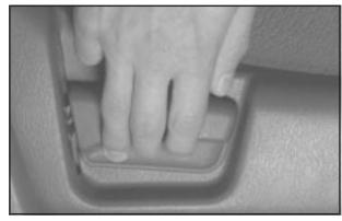
To adjust the seatback, lift the lever on the outboard side of the seat cushion. Release the lever to lock the seatback where you want it. Pull up on the lever, and the seatback will go to the upright position.
